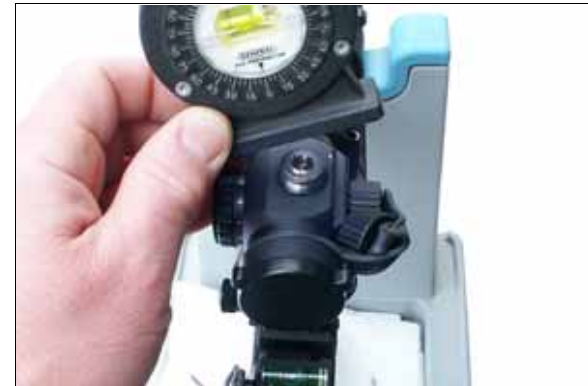
10. Remove the top elevation adjustment cover, and place a level on the exposed flat surface.
