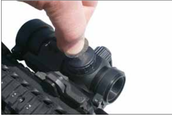
The Mark III uses a flat 3 volt CR2032 battery, which is easily changed with a coin. Carry extra batteries !!!
